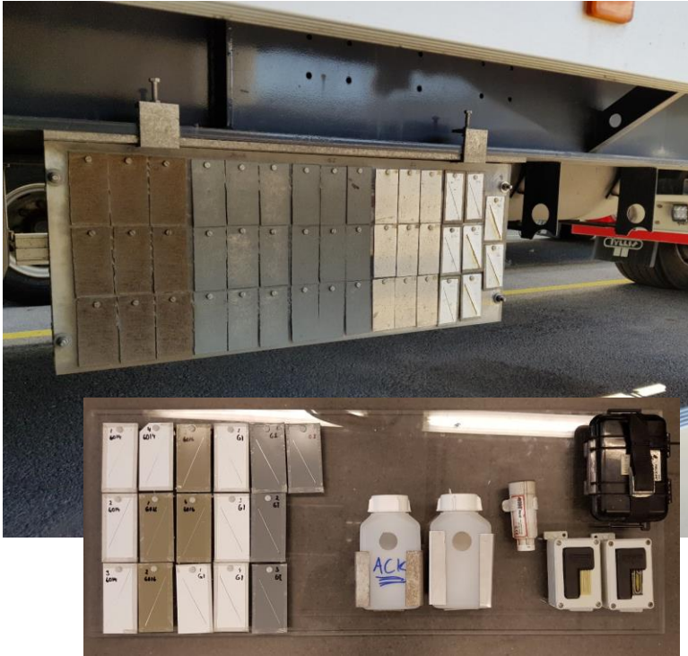
Mobile corrosion test for automotive materials 2022-04-06
