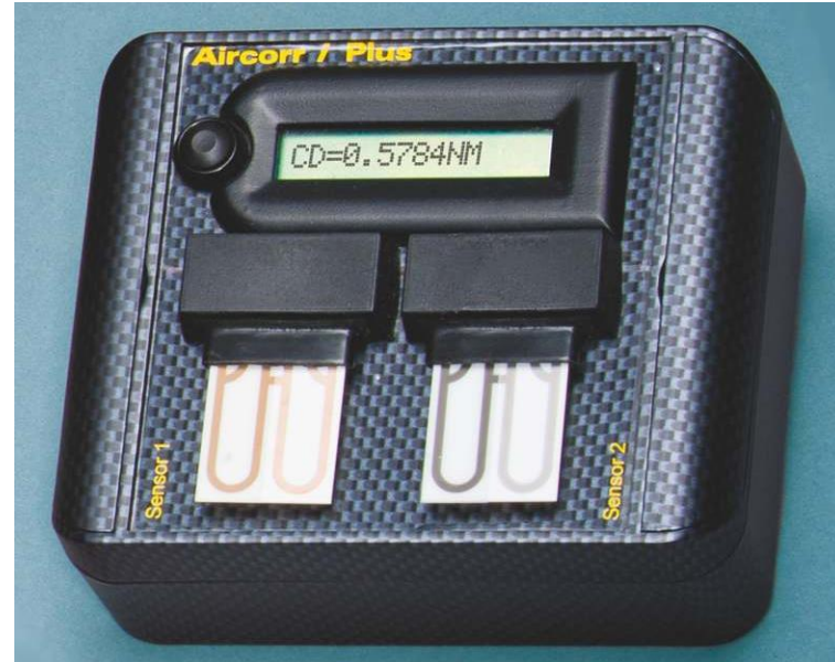
AirCorr I Plus: Indoor version with temperature and RH sensors, 2 exchangeable corrosion sensors, LCD showing actual corrosivity
