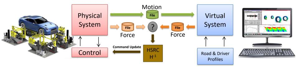
HSRC converges on the 6 Degree of Freedom (DOF) force & motion solution at each corner that simultaneously solves for the unique solution of the complete, coupled system at each hybrid interface.
