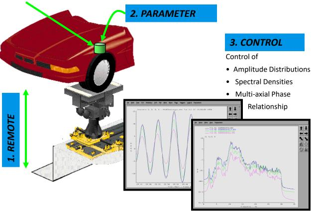
Remote Parameter Control (RPC) is an advanced simulation technique used to repeatedly replicate and analyze "in service" vibrations and motions of a specimen using a dynamic mechanical system in a controlled laboratory environment.
