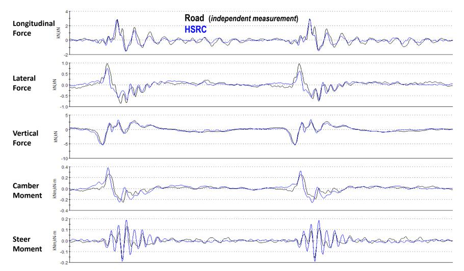
■ With accurate tyre models and road scans, HSRC produces loads statistically consistent with measured road data → Accurate tests without RLDA!
