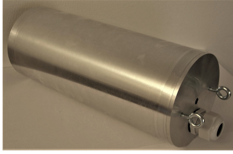
Fig 5.3: Cylindrical test object with cable entity and loops for fastening.
