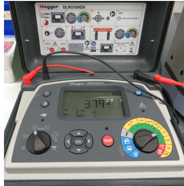
Megger mikroohm measurement unit with 2 voltage probes and 2 current probes
