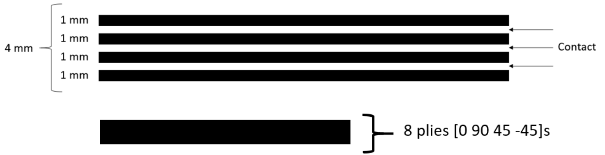
Figure 3.2: The cross section of the model with four layers, each containing 8 plies.
