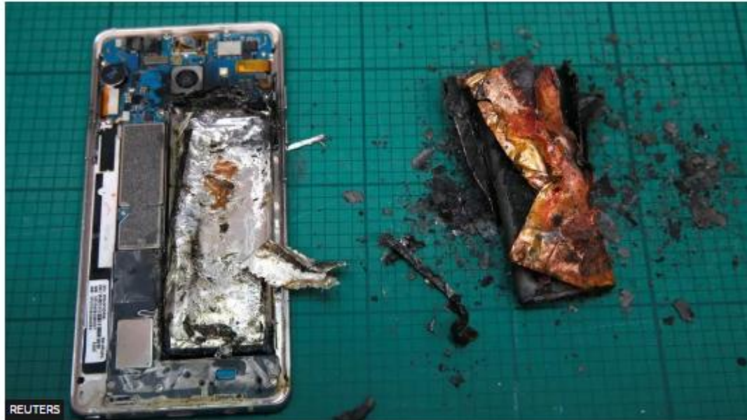
A Samsung Note 7 handset caught fire during a lab test in Singapore
